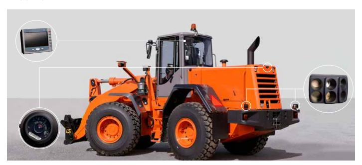
The combination of sensors and camera(s) offers the operator both passive and active safety information about the free space in the surroundings of the machine.
